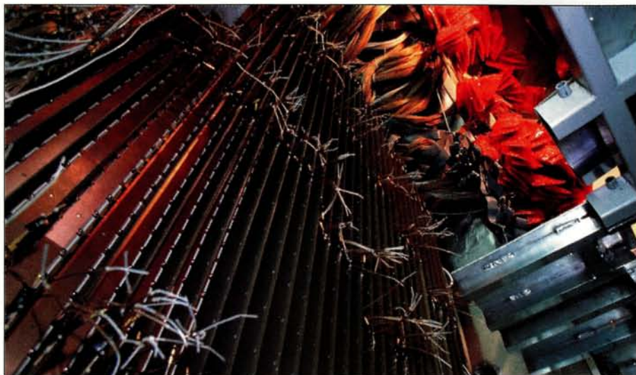
Detail of electronics installation for readout from the liquid krypton calorimeter of the NA48 experiment at CERN, prior to being hidden from view inside the cryostat.
